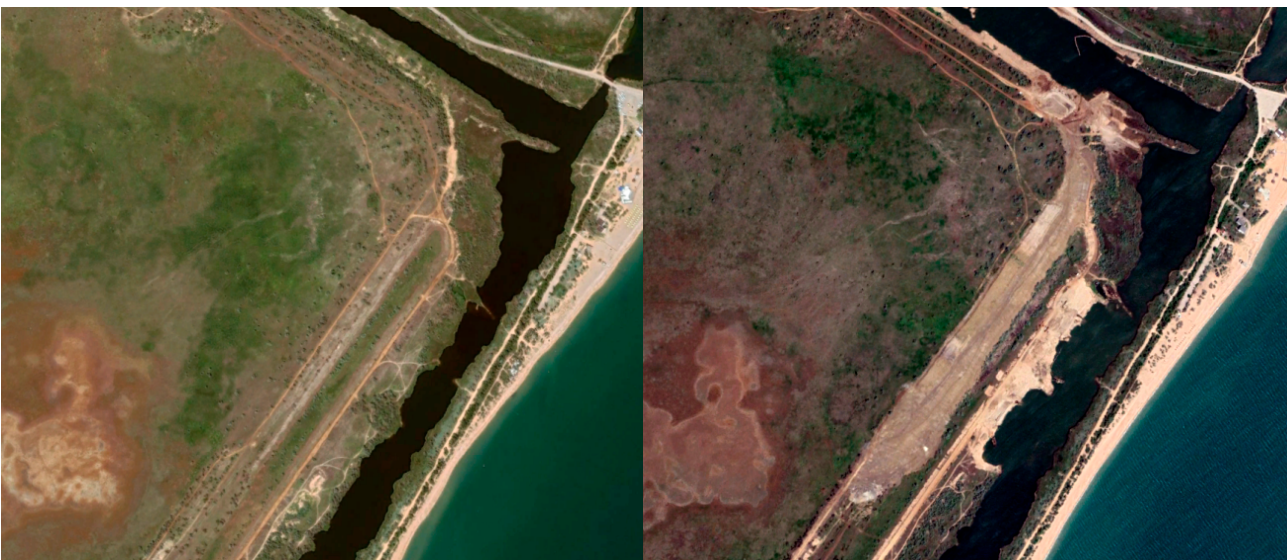
Fig. 18-19. Sand excavation from the tailings dam in satellite photographs from 2013 (left) and 2019 (right). Source: KrymSOS .
